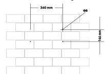
2. Drill holes and fix the mounting plate to the wall. Mount the inverter to the plate.
